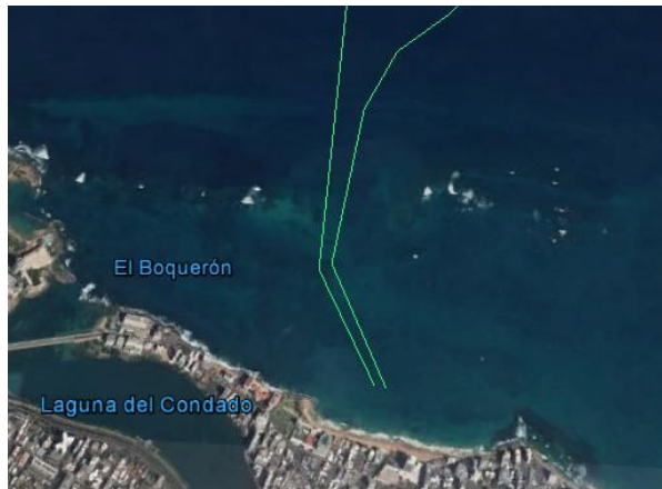
Fig.3 Global Marine GIS mapping with possible coaxial submarine cables out of the Condado area in San Juan, Puerto Rico.
